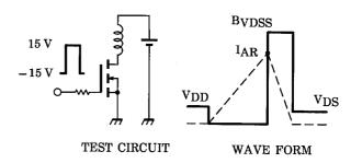
$$\begin{aligned} R_G &= 25~\Omega \\ V_{DD} &= 90~V,~L = 594~mH \end{aligned} \qquad EAS &= \frac{1}{2} \cdot L \cdot I^2 \cdot \left( \frac{BVDSS}{BVDSS - VDD} \right) \end{aligned}$$
